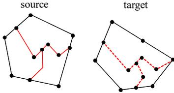
Figure 2. Examples of representing a source and a target by points and lines. The black and red lines represent the object outlines and the cracks, respectively.
